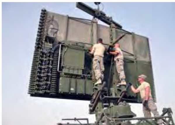
Figure 9–24: Members of 72th EACS installed A/N-75 Air Surveillance Radar at an undisclosed SWA location; source of non-traditional weather data. (USAF photo by 1Lt Victoria Porto)
