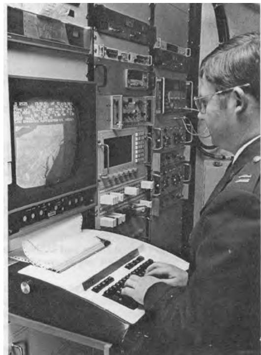
Figure 6-8: Meteorological Satellite Coordinator operating the AN/TMQ-35 MARK IV DMSP satellite readout van, 1981.
