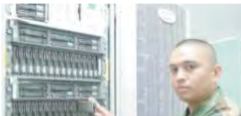
Figure-1-14: SSgt Jay Sablan, AFWA Communications Directorate, Network Systems Administrator, replaces a failed hard drive on an AFWA server.
