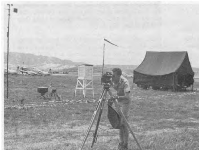
Figure 3-7: 1Lt Albert T. Watson, Jr., readying Pibal run at advanced F-51 strip in Korea, late 1950. In background (left to right) are AN/GMQ-1 Wind Equipment, AN/TMQ-2 Ceiling Light Set, and ML-41 Shelter protecting ML-24 Psychrometers (dry bulb and wet bulb thermometers)
