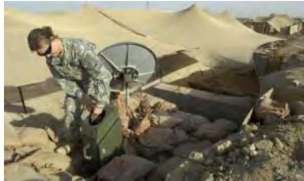
Figure 9-1: TSgt. Andrea Patterson, assigned to Forward Operating Base Kalsu south of Baghdad, Iraq, cleans debris from the lens cover on the cloud height detector of the AN/TMQ-53.
