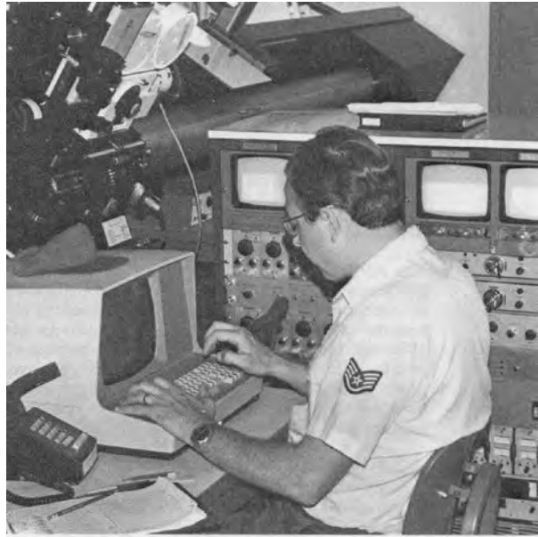
Figure 6-3: SSgt Mike Springer (Det 7, 2WS, Holloman AFB, NM) using a control unit of the AN/FMQ-7 Solar Optical Telescope. When combined with an AN/FRR-95 an observatory became part of the Solar Electro-optical Observing Network (SEON)
