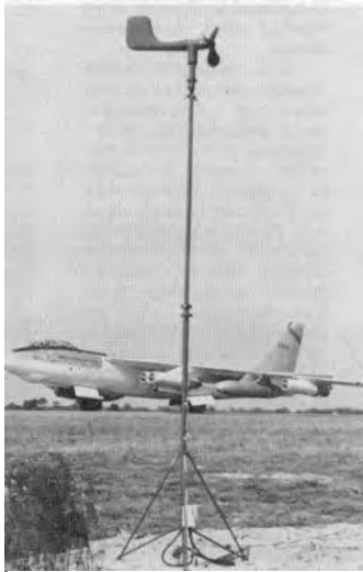
Figure 3-12: T-420 Wind Direction and Speed Transmitter, a subsystem of the AN/GMQ-11 Surface Wind Set.
