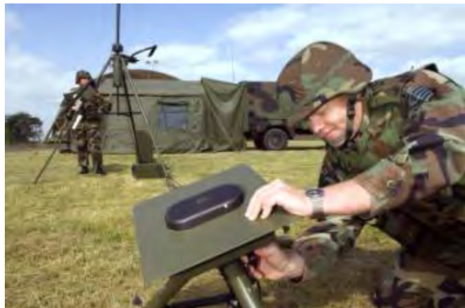
Figure 8-2: SSgt Craig Gaillardet attaches the lightning detector to the base unit of the AN/TMQ-53 Tactical Meteorological Observing System (TMOS). Sergeant Gaillardet, a combat weather forecaster with the 7th WS, and other members of his team conduct realistic training to optimize support to their supported US Army unit. (USAF photo by MSgt John E. Lasky)
