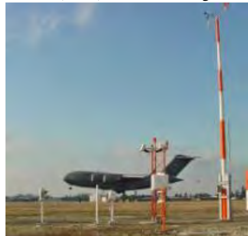
Figure 8-15. A C-17 Globemaster III aircraft at AFWA, 24 May 2003. AFB, WA as the AN/FMQ-19 Automatic Meteorological Station creates an automated surface weather observation. Located near the touchdown point of the runway, primary sensors visible are, from left, precipitation, lightning detection, cloud height, combined visibility/present weather, and wind direction/speed [atop
