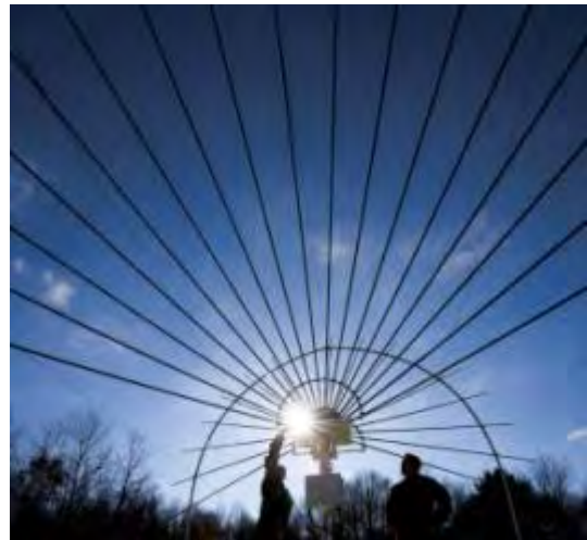
Figure 9-12: Solar Radio Spectrometer (SRS) dipole antenna at Sagamore Hill Solar Radio Observatory, MA. The SRS is a key component of the Solar Electro-Optical Observing Network (SEON)
