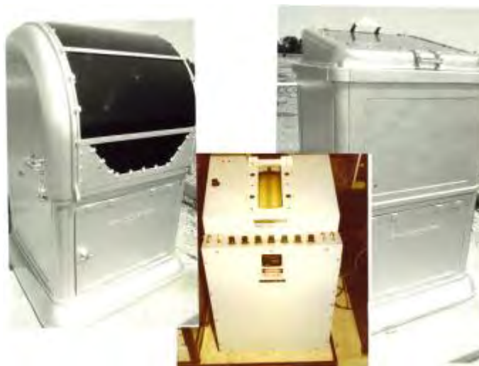
Figure 4-3: AN/GMQ-13 Cloud Height Set, ML-506 Projector (L), IP-327 Indicator (C), and ML-507 Detector (R); more frequently referred to as Rotating Beam Ceilometer (RBC) because of the rotating light beam technology used in the projector.
