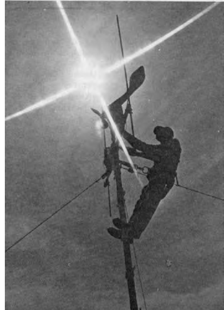
Figure 6-1: A weather equipment repairman aligns a T-755 Wind Sensor, a sub-system of the A/N-GMQ-20 Wind Set.
