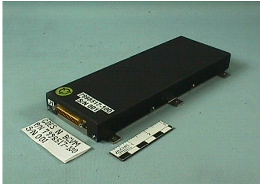
Figure 10-6. Battery Cell Voltage Monitor
