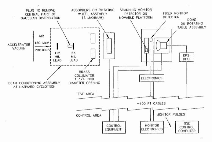
Figure 2.1. DOME Sensor Calibration Configuration at the Harvard Cyclotron.
