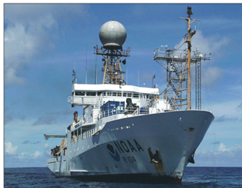
NOAA Ship Ronald H. Brown is a multipurpose research vessel capable of supporting physical, chemical, and biological oceanography; atmospheric and climate research; marine acoustics; marine geology and geophysics; bathymetry; and a host of multidisciplinary environmental investigations in coastal and deep ocean regions.
