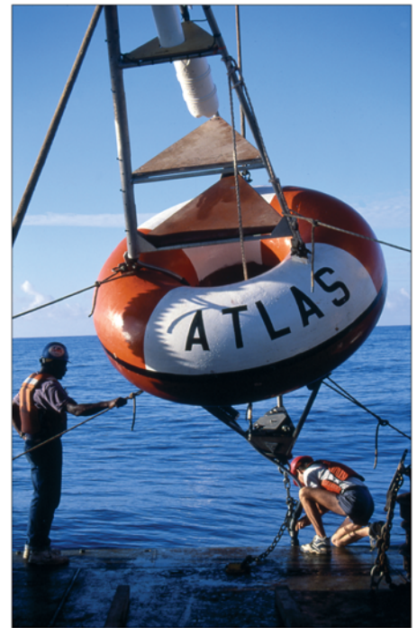
Deployment of a Tropical Atmosphere Ocean (TAO) buoy. These buoys are anchored to the ocean floor at depths ranging from 2000 to 5000 meters.
