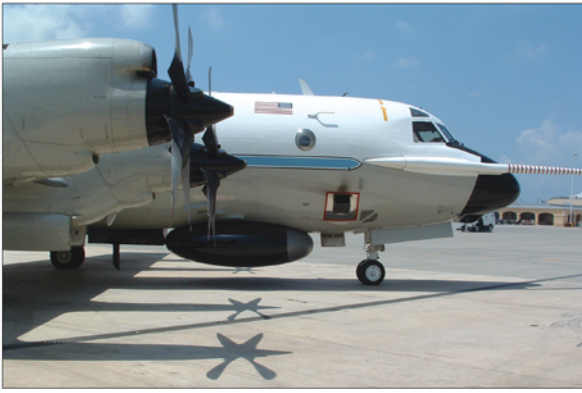
NOAA WP-3D Orion on the tarmac. WP-3D are equipped with scientific instrumentation, radars, and recording systems for both in situ and remote sensing measurements of the atmosphere, Earth, and its environment. These aircraft are on standby or deployed for hurricane research and reconnaissance 120 days each year.
